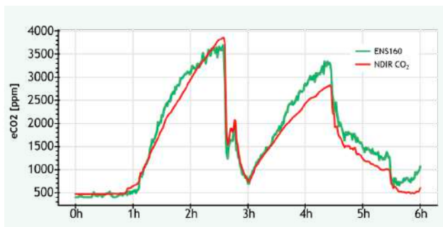
Figure 3: Comparison between ScioSense ENS160 eCO 2 readings and NDIR CO 2 outputs.
